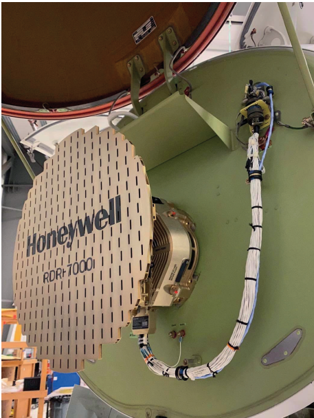
Radar image of mounted RDR-7000 in place of former radar system
