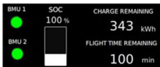
Fig. 14 Crew Alerting System
