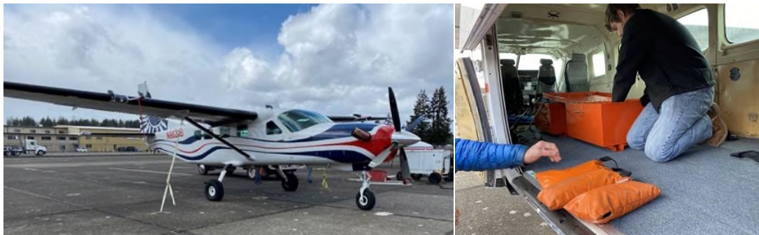
Figure 21 – Rental Caravan and Ballast System
