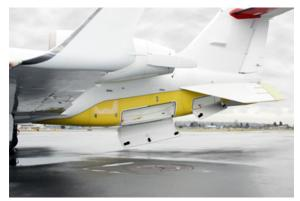
Lear 60 Aft Fuselage Locker shows its two connected baggage compartments. Both are full-width and depth for almost 30 cubic feet additional cargo space.
